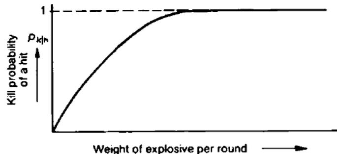
Figure 119. *Relationship between the kill probability of a hit and the weight of explosive per round.*
